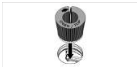
Fig. 8.8 Inserting the activated charcoal filter through the vent opening
